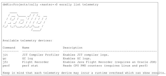
You can attach one or more of these telemetry devices to the benchmarked cluster. However, this only works if Rally provisions the cluster (i.e. it does not work with --pipeline=benchmark-only).
